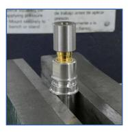
10. Using a drill press or arbor press, push the Contact into the Connector Shell. Press until the Contact is pressed completely into the Connector Shell (left: male, right: female).
