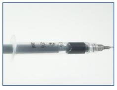
15. Insert the syringe with needle deep into the Connector Shell. Inject the epoxy into the Connector Shell until the epoxy starts to come out the rear of the Connector Shell. Move the cable around inside the Connector Shell to ensure that both the outer surface of the cable jacket and the inner
