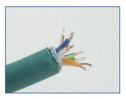
5. Insert the wires into the contacts on the Connector Insert and solder them in place. It is very important to make a clean solder joint with minimal solder outside the joint – excess solder can cause shorts between the wires or between a wire and the Connector Shell. Double-check that each wire is soldered to the correct contact (the pinout will depend on the particular application).
