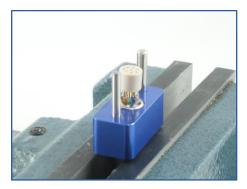
10. Slide the upper half of the Termination Tool onto the lower half of the Termination Tool. Insert the pins on the upper half of the Termination Tool into the contacts on the Connector Insert, rotating the Connector Insert as necessary to ensure the proper pinout for your application (make sure that the wires are in the desired alignment relative to the flat on the Connector Shell).
