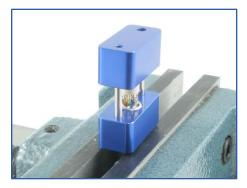
11. Using a drill press, push down on the upper half of the Termination Tool until the Connector Insert is pressed completely into the Connector Shell.
