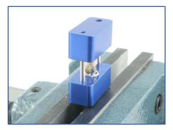
11. Using a drill press, push down on the upper half of the Termination Tool until the Connector Insert is pressed completely into the Connector Shell.
