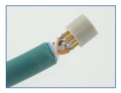
6. Abrade the last 3 cm of the cable jacket with sandpaper and clean with a paper towel that has been slightly moistened with acetone to prepare it for potting. From this point on, be careful to keep this part of the cable jacket clean.
