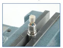
9. Place the lower half of the Termination Tool over the Connector Shell, aligning the flats.
