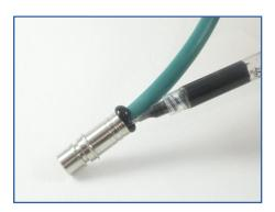
17. Clean off the excess epoxy with a paper towel and acetone or alcohol.
